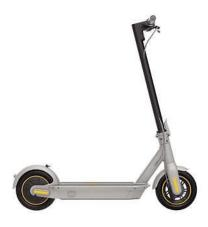
Apart from the outstanding design, the new Ninebot MAX G30LP is designed to be sturdier and even more powerful. This fold-up design includes 10-inch pneumatic tires, built-in front LED lights, 18.6 max speed, 25 mile range, 20% hill grade, IPX5 water-resistant, and a 367Wh battery.
