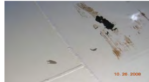
Transport Damage on New Second-Generation IMM
