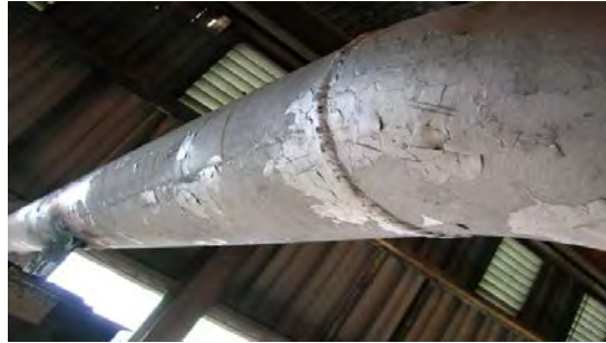
Thin Film Silicone Applied too Thickly
