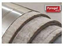
Pyrogel HPS is optimized for hightemperature pipe and vessel applications in the refining, chemical processing, and power generation markets. With its extremely low thermal conductivity at high temperatures, Pyrogel HPS based solutions can be up to 75% thinner than available insulation materials. As a result, Pyrogel HPS is suitable for installation in congested areas or near mechani-
